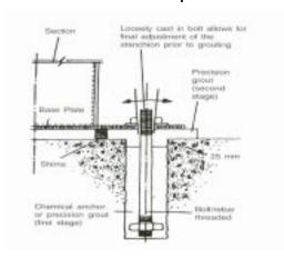
The compressive strength of the grout must exceed 50 N/mm<sup>2</sup> at 7 days and 60 N/mm<sup>2</sup> at 28 days.
