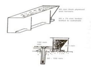
Pouring should be from one side of the void to eliminate any air or presoaked water becoming trapped under the base plate. It is advisable to pour the grout across the shortest distance of travel. The grout head must be maintained at all times so that a continuous grout front is achieved.
